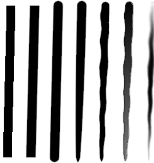
Figure 8 The cumulative effects of adding stroke operations, from left to right: raw stroke, antialiasing, taper, flare, wiggle, alpha fade, and texture-mapping.
