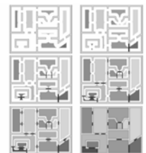
Figure 4: Different steps of the watershed algorithm. Two catchment basins getting in contact during an iteration reveal the presence of an opening: a portal is built to separate them.
